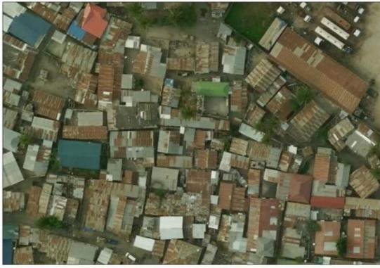
Figure 4.22: Buildings crowding reduce vehicular mobility, privacy and impose settlement in danger in case of fire outbreak
