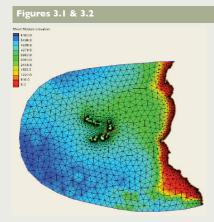
Figures 3.1 The ADCIRC storm surge model was installed and run for the Cape Verde islands, the model catchment was quite large (Figure 3.1).
