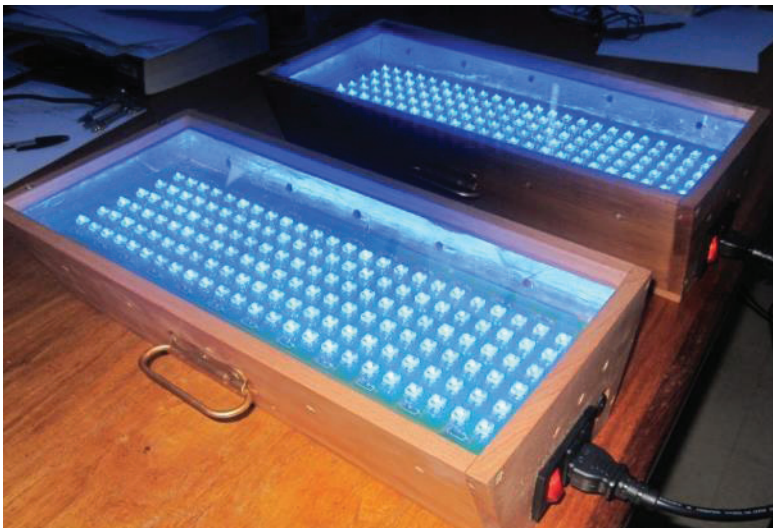
Figure 5.7: Phototherapy box photographs at lowest level of irradiance
