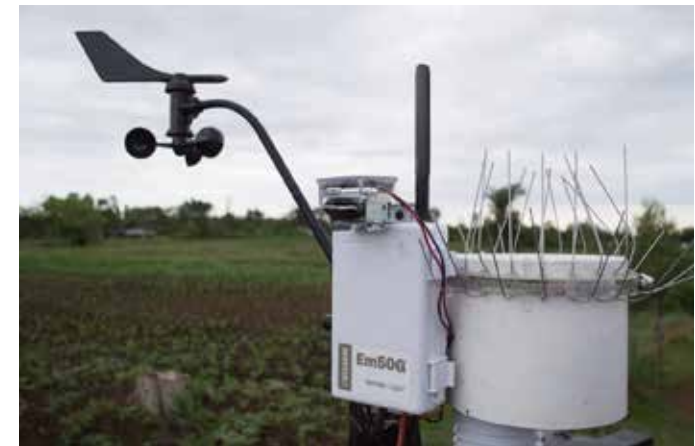
A Trans-African Hydro-Meteorological Observatory (TAHMO) weather station in Lela, Southwestern Kenya. With an eye on the weather, farmers rely on the crops they grow. Photo © ECA
