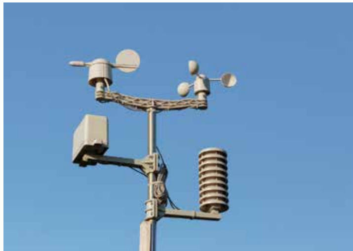
A weather station comprising of sensors for wind speed, wind direction, rain and temperature. In July 2017, the African Climate Policy Centre launched the second phase of the Weather and Climate Information Services for Africa (WISER), to be implemented within a span of three years. Photo Courtesy
